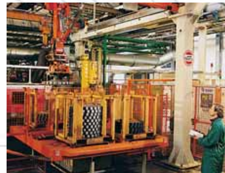
Heat treating automated station
