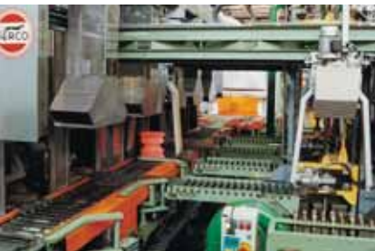
Through hardening furnace
