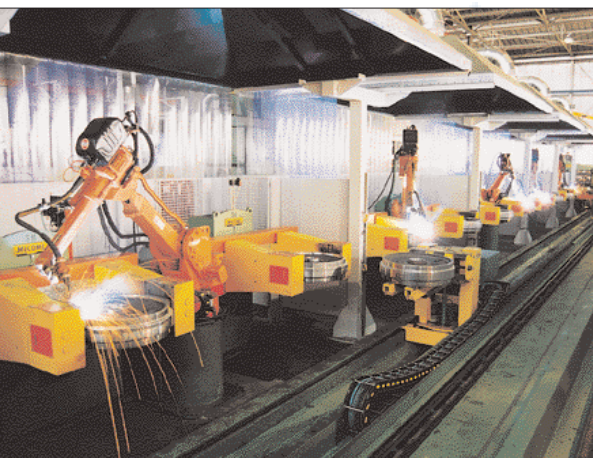
▲ Automated welding line
