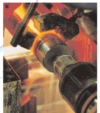
Induction hardening of shafts
