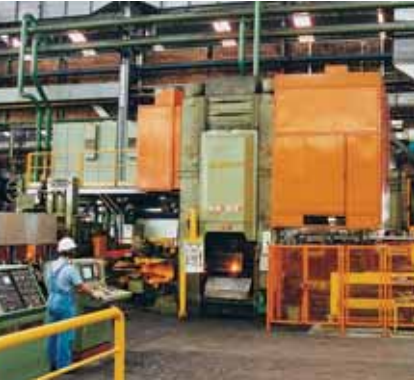
Track links forging
