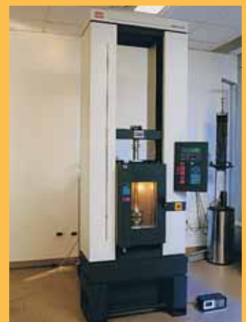
Stress analysis at extreme temperatures
