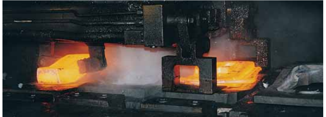
Track links forging
