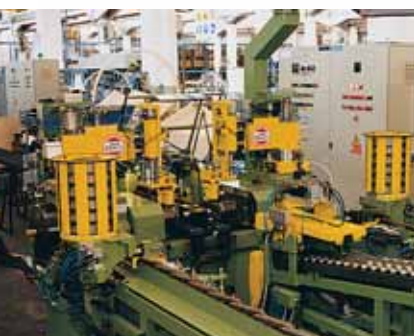
▼ Track chains fully automated assembly
